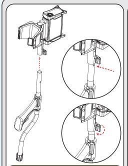
Holding the metal pin pressed, insert the S-rod into its place underneath the system box and secure it by tightening the wingnut as shown in the picture.
