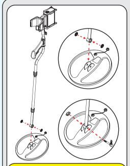
Place the washers into the openings on both sides at the end of the extension shaft. After placing the shaft on the coil as shown in the picture, insert the fastening screw through the hole and tighten it using the wingnut.
