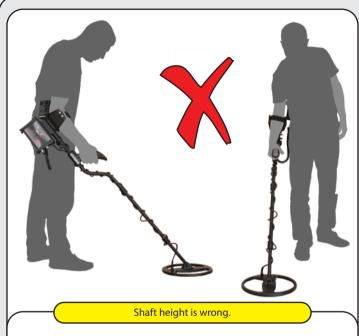
It is very important to adjust the shaft to your height correctly to be able to search without discomfort and fatigue.
