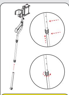
Insert the extension shaft into the upper shaft holding the metal pin pressed and adjust the height by clicking the pin into one of the holes. Then, secure it by tightening the twist lock again.
