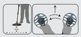
After the settings are adjusted, you can start searching by lifting the search coil 5cm. above the ground and sweeping it right and left, keeping it parallel to the ground.
