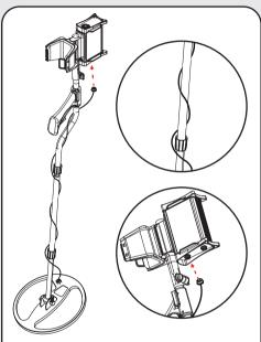
Wrap the coil cable around the shaft all the way up as shown in the picture and after inserting it in the coil input socket underneath the system box, secure it by twisting the connector. Pay attention to not wrap the cable too tight during this step.
