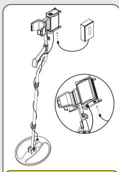
Plug the battery cable into the battery input socket underneath the system box and tighten securely.
