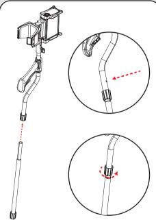
Again by holding the metal pin pressed, insert the upper shaft into the S-rod and click the pin into its hole. Then, secure it by tightening the twist lock.
