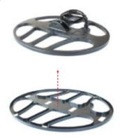
Coil cover use is optional. It protects the search coil from scratches. If you want to use the cover, remove the protective sheets from the tapes inside the cover, attach the cover to the coil and press firmly to make them stick together. Once the cover is attached, you cannot take it off.
