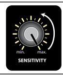
If the detector emits false signals due to interference, reduce the sensitivity until the signals go away and start searching.
