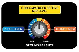
Golden Sense ground balance setting consists of 3 different levels:
