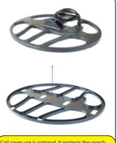
Coil cover use is optional. It protects the search coil from scratches. If you want to use the cover, remove the protective sheets from the tapes inside the cover, attach the cover to the coil and press firmly to make them stick together. Once the cover is attached, you cannot take it off.
