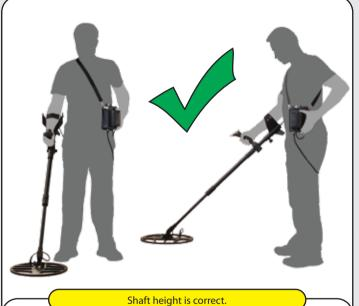
Adjust the height of the shaft so that you are standing in an upright position, your arm is relaxed and the search coil is approximately 5cm (~2") above the ground.
